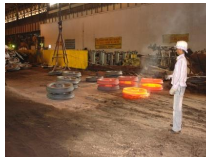
Fig.5 Rolling of wheel in Wheel Mill and final wheel after forging
