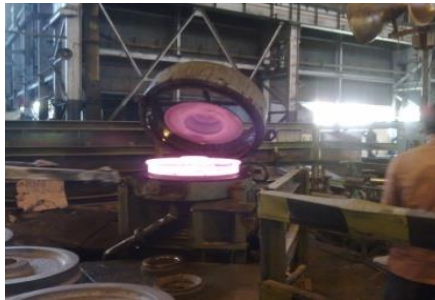
Fig.8 Heat Treatment of wheeland stacking of Heat Treated black wheels
