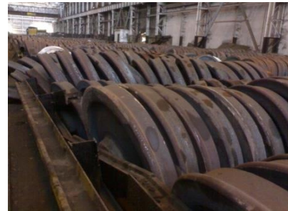
Fig.8 Heat Treatment of wheeland stacking of Heat Treated black wheels
