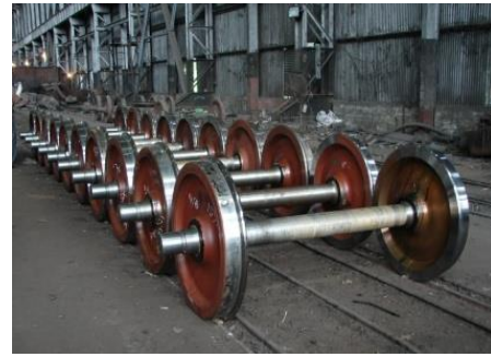
Fig.10 Tested OK loose wheel and assembled wheel sets ready for despatch
